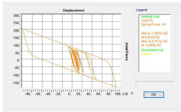
Figure 20: Lead Rubber Bearing's hysteresis loop for K_V = 9653702 \text{ kN/m} .
