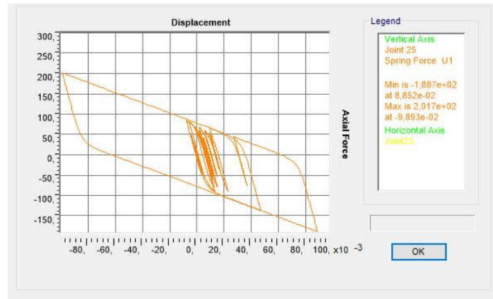
Figure 17: Lead Rubber Bearing's hysteresis loop for K_V = 8653702 \text{ kN/m} .
