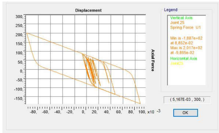
Figure 8: Lead Rubber Bearing's hysteresis loop for K_V = 5653702 \text{ kN/m} .
